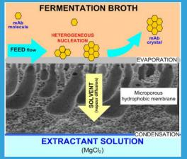
BIOPURE will provide a breakthrough advancement in terms of productivity efficiency via continuous manufacturing, cost reduction, process intensification, and enhanced environmental sustainability avoiding extensive use of chemicals, compared to the standard processes (i.e., chromatography-based platforms).
